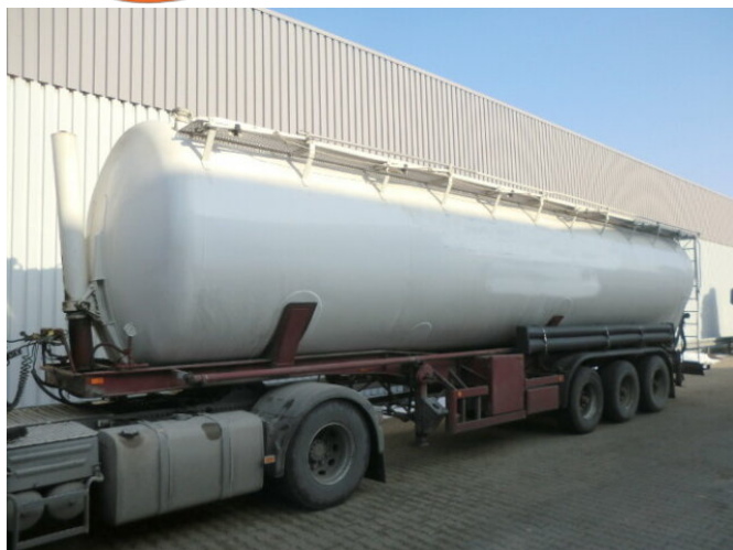
KAESSBOHRER SSK 56/10-24, Kippsilo ca. 56m 3
